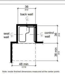
FIGURE 11B-608.2.1 TRANSFER TYPE SHOWER COMPARTMENT SIZE AND CLEARANCE
